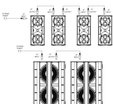
11. Fig. Parallel connection for the X102FD and XW218 (mains). Do not connect more than four units of X102FD units two of XW218 using the AC Mains link connector.
