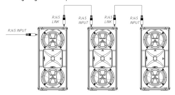
**Fig.9.** Parallel connection for the X102FD (network). You can link up to eight units when using Dante networking, or more when not using it.
