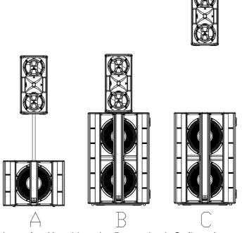
Fig. 15. X102FD with subwoofer (A: with pole, B: stacked, C: flown)
