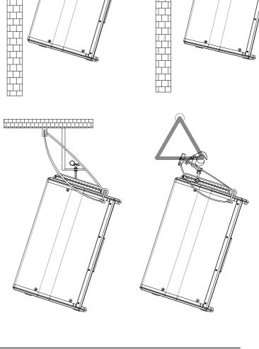
Fig. 23. Flying of one unit X102FD with RB-L and RB-L/GT
