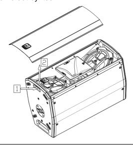
• Pull the horn and turn it 90°. We recommend you to put your hands on points "1" and "2" to make the process easy (edge of the horn)
