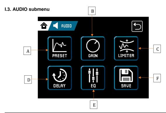
A. **Preset**: Selection of factory sound presets. The available factory presets depend on each model and can be found on each model user manual.
