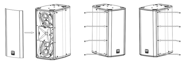
• Insert the grille through the slots of the side metal profiles (1) (2).
