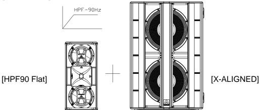
Fig. 4. Preset [HPF90 Flat] configuration
