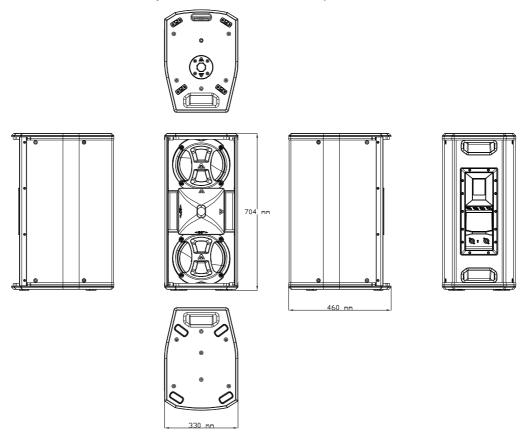
Fig. 1. X102FD external dimensions
