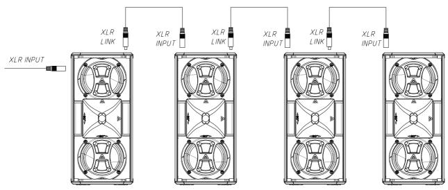
Fig. 7. Parallel connection for the X102FD (signal)
